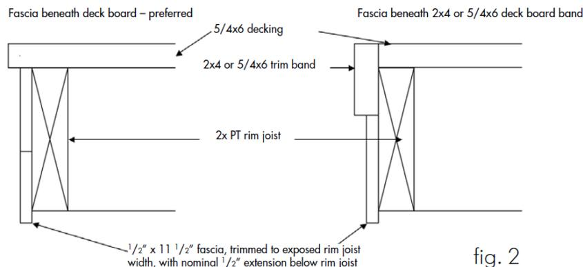
Note: When using fascia to cover joists wider than 11 ½" (292 mm), either stack multiple layers of fascia or use a combination of fascia boards, deck boards and 2x4s as accents to create a unique look. (fig. 2)
